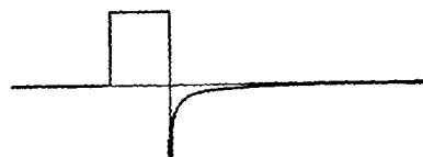
FIG. 3-25.—Spike often produced by shunt capacity.
