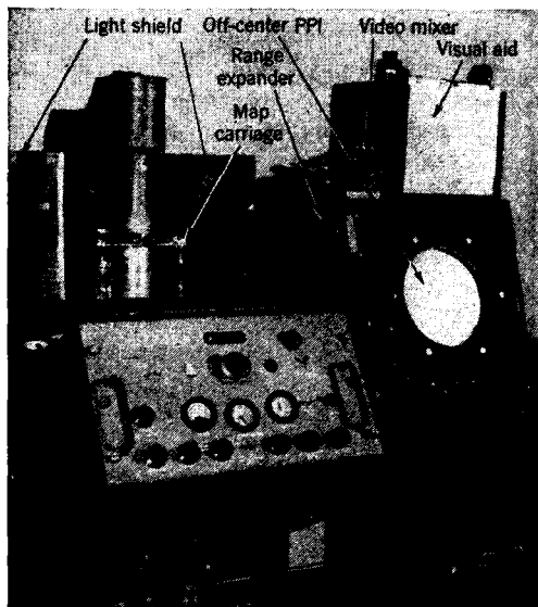
FIG. 7-51.—A typical video-mapping installation using a converted Emerson trainer.
