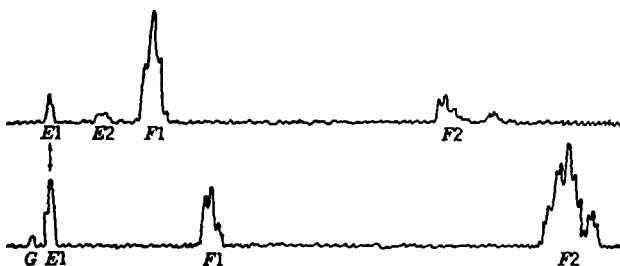
FIG. 3-20.—Pulse trains from a pair of stations approximately matched for sky-wave readings.
