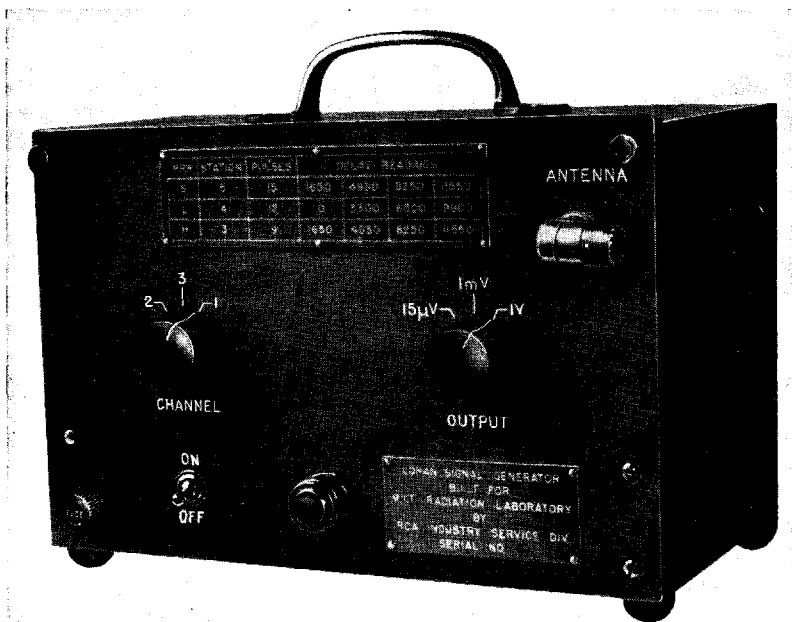
FIG. 11-18.—Pulse-signal generator for testing receiver-indicator.
