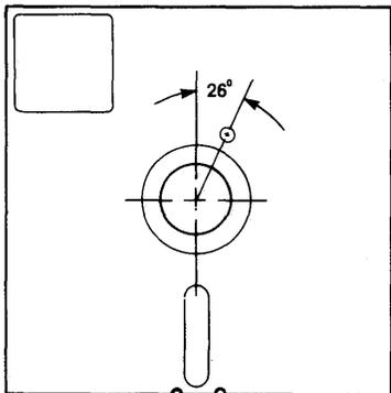
The index hole for 3M DS-DD diskettes is located at approximately 26°.
