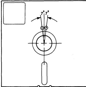
The index holes for 3M SS-SD-R and SS-DD-R-128/F reversible diskettes are located at approximately 7° on each side.
