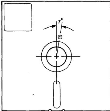
The index hole for 3M SS-SD and SS-DD diskettes is located at approximately 7°.
