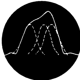
C. Center Frequency Coil Tuned to High End of I-F Response
