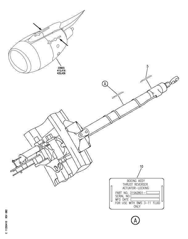
ACTUATOR ASSY-LOCKING UPR (PLACARDS AND MARKINGS ONLY) FIGURE 10
