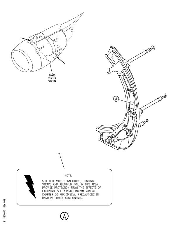
WIRING INSTL-THRUST REVERSER (PLACARDS AND MARKINGS ONLY) FIGURE 5
