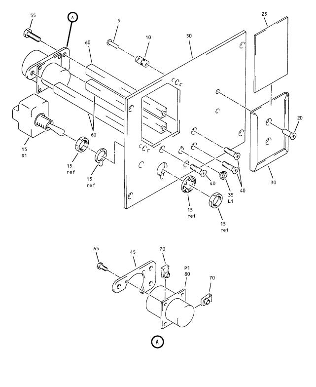
Broadcast Radio Control Module Assembly IPL Figure 1
