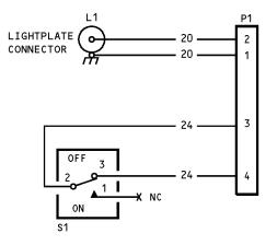
69-76497-1 Broadcast Radio Control Module Assembly Schematic Diagram Figure 101
