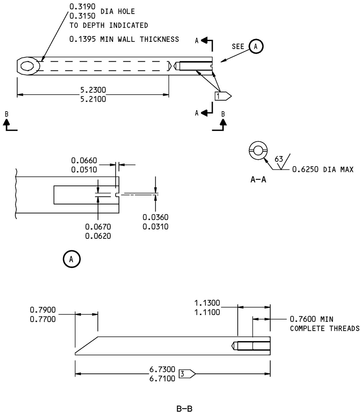
141A6810-1 Latch Pin Assembly Repair
