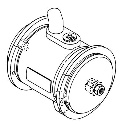
Standby Hydraulic System Reservoir Assembly Figure 1
