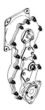
Aft Airstairs Mechanism Reduction Gearbox Assembly Figure 1
