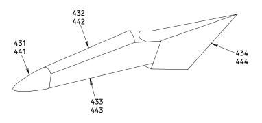
SUBZONE 430 - NO. 1 NACELLE STRUT SUBZONE 440 - NO. 2 NACELLE STRUT
