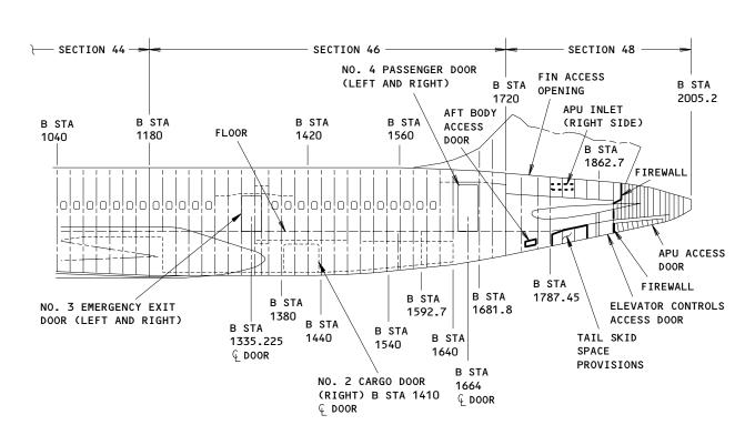
Body Station Diagram Figure 201 (Sheet 1)
