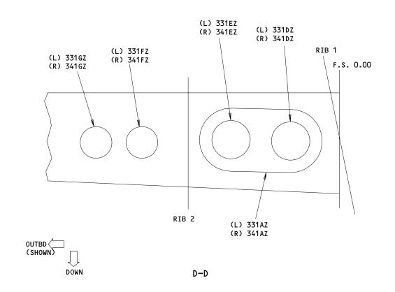
Sub-Zones 330/340 Access Doors and Panels Figure 203 (Sheet 2)
