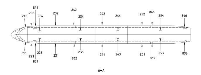
Upper Half of Fuselage Zone Diagram Figure 203
