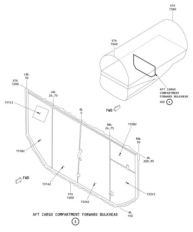
Aft Cargo Compartment Forward Bulkhead Figure 202
