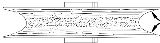
PULLEY NOT ALIGNED CORRECTLY
