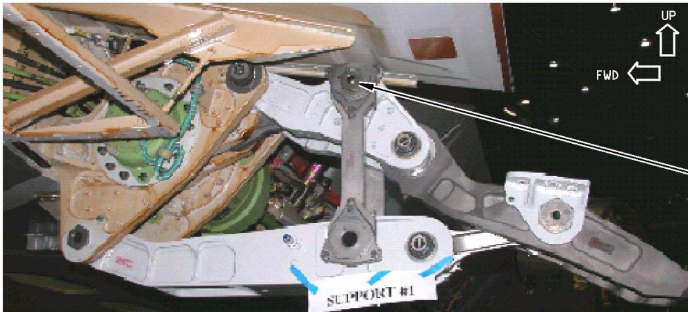
VIEW OF FLAP SUPPORT NO. 1 IN THE EXTENDED POSITION
