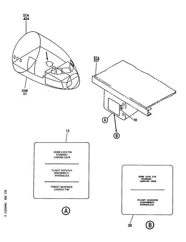
BOX ASSY-LG DOWN LOCK PIN (PLACARDS AND MARKINGS ONLY) FIGURE 1
