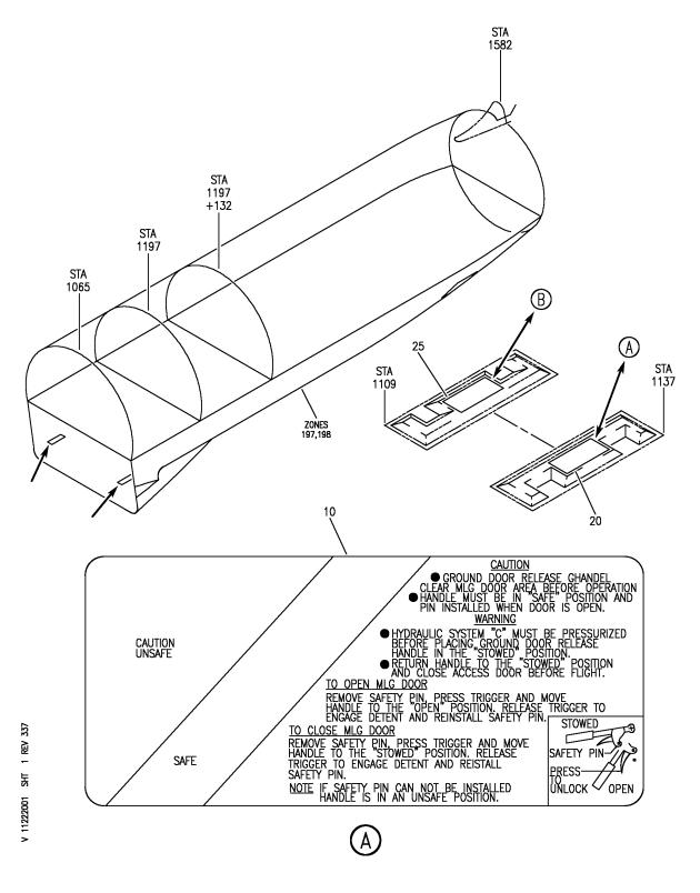
DOOR ASSY-AFT FAIRING MLG GND CONT ACCESS (PLACARDS AND MARKINGS ONLY)
