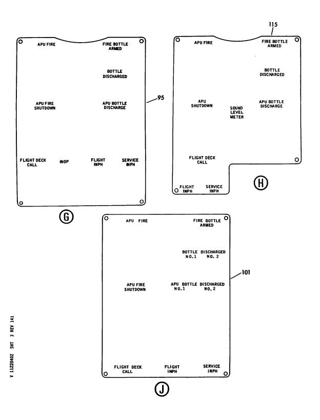
PANEL ASSY-APU SHUTDOWN P40 (PLACARDS AND MARKINGS ONLY) FIGURE 2 (SHEET 3)
