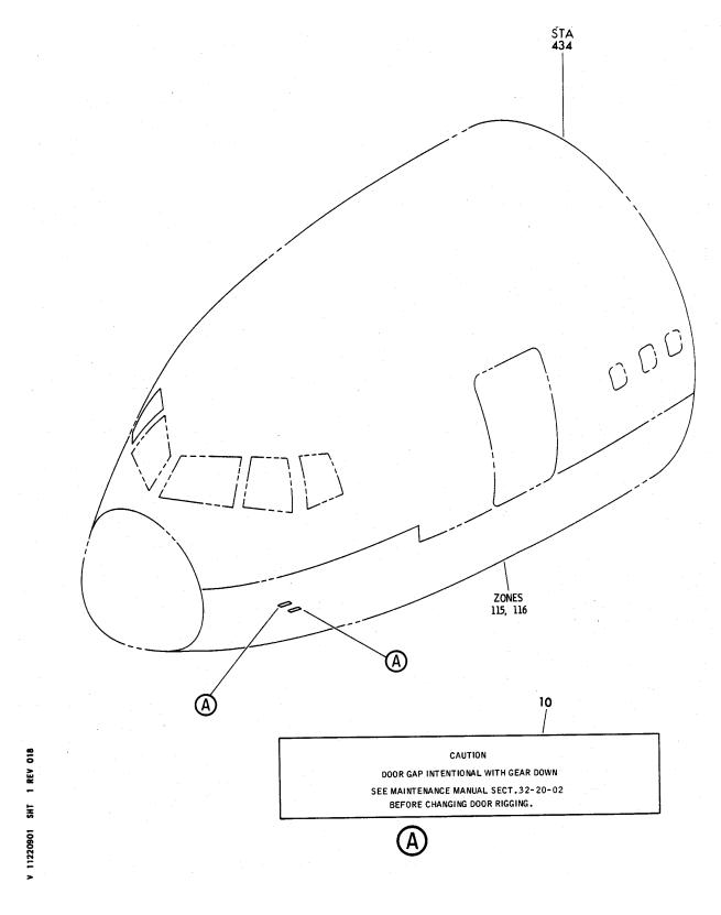
MECHANISM INSTL-NLG FWD DOOR OPERATING (PLACARDS AND MARKINGS ONLY) FIGURE 1
