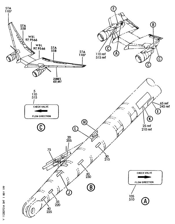
HYDRAULIC INSTL-SECT. 31 ENG FAIRING AFT (PLACARDS AND MARKINGS ONLY) FIGURE 1A (SHEET 1)
