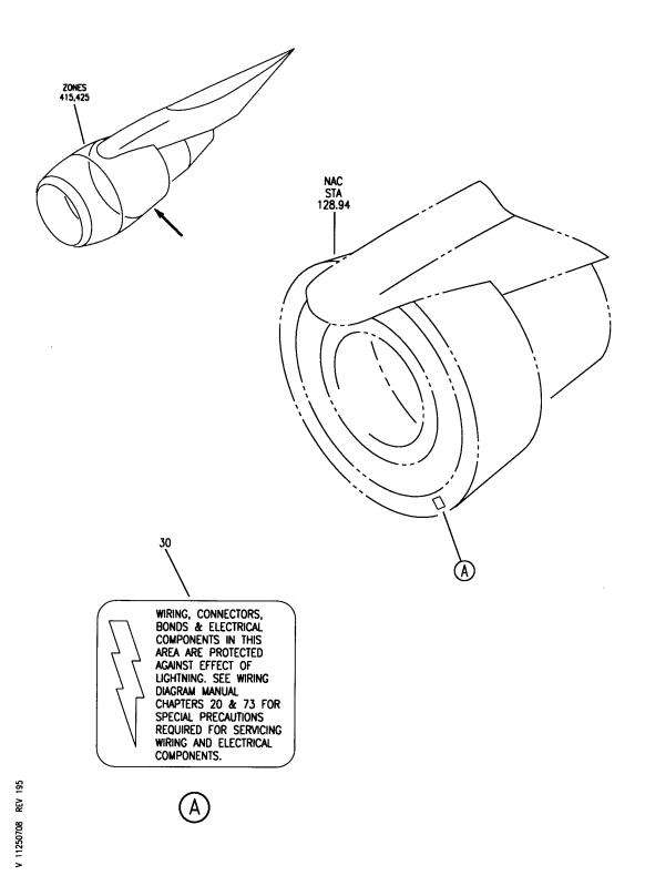
COWL ASSY-FAN DUCT (PLACARDS AND MARKINGS ONLY) FIGURE 8
