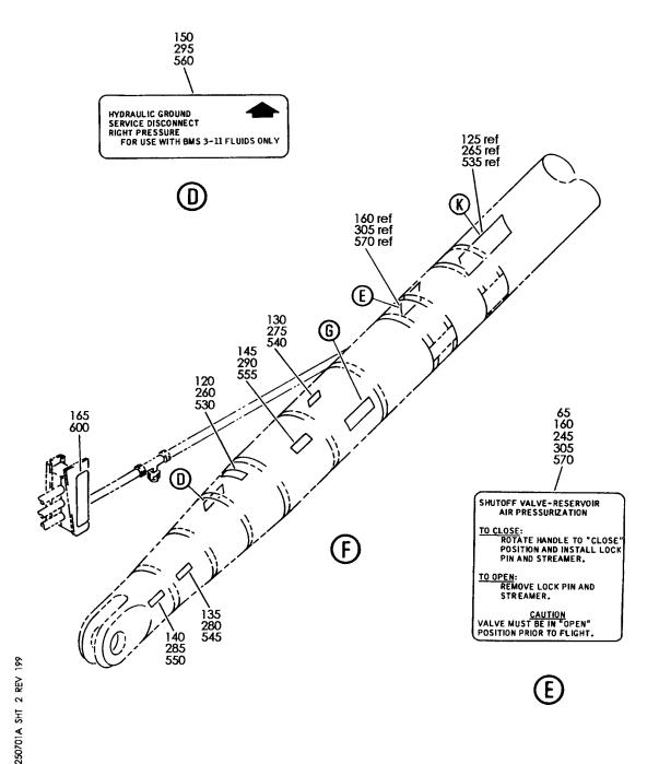
HYDRAULIC INSTL-SECT. 31 ENG FAIRING AFT (PLACARDS AND MARKINGS ONLY) FIGURE 1A (SHEET 2)
