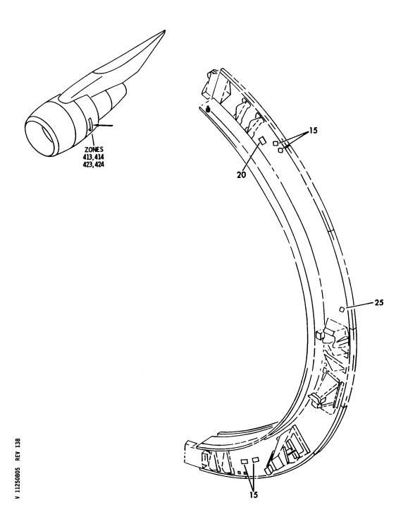
COWL ASSY-FAN DUCT (PLACARDS AND MARKINGS ONLY) FIGURE 5
