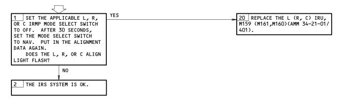
Entry INOP to Single IRS (Align Flashes After Second Entry). Position Entry from FMC-CDU Unsuccessful. Figure 105A
