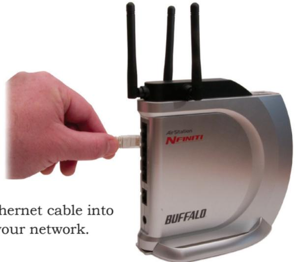
Plug the other end of the Ethernet cable into a hub, router, or switch in your network.
