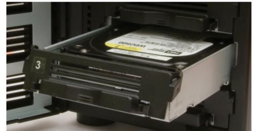
Lower the drive carefully to the work surface.
