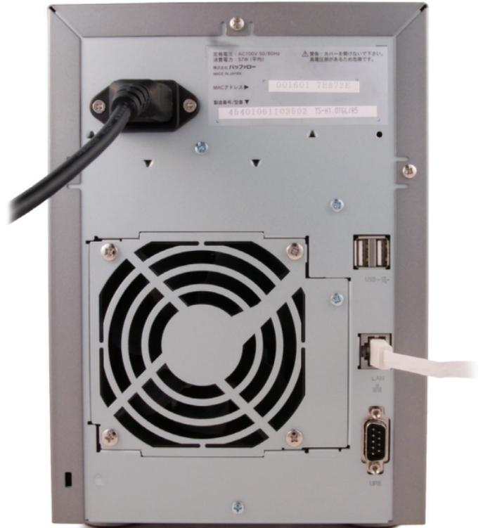
Begin setting up your TeraStation by plugging your *power cable* and *Ethernet cable* into the back of the TeraStation as shown.
