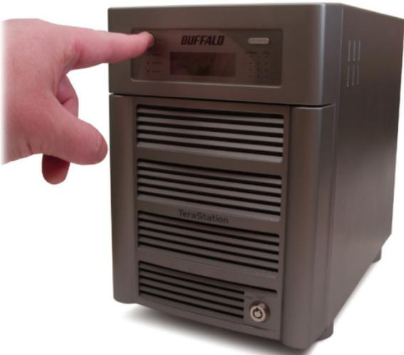
Press the *power button* on the front panel. LEDs will light as your TeraStation boots up.
