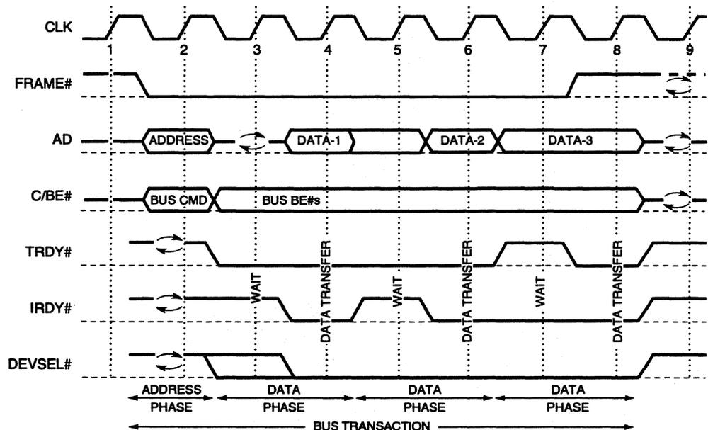
Figure 2-4. Basic Read Operation
