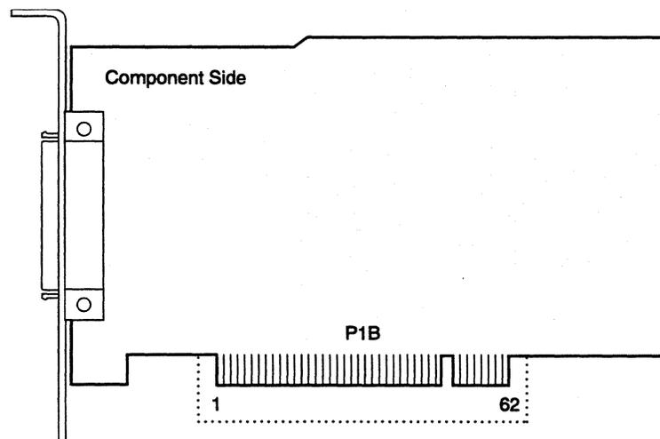
Figure 2-3. Connector Rows on the PCI Host Adapter's Board Edge
