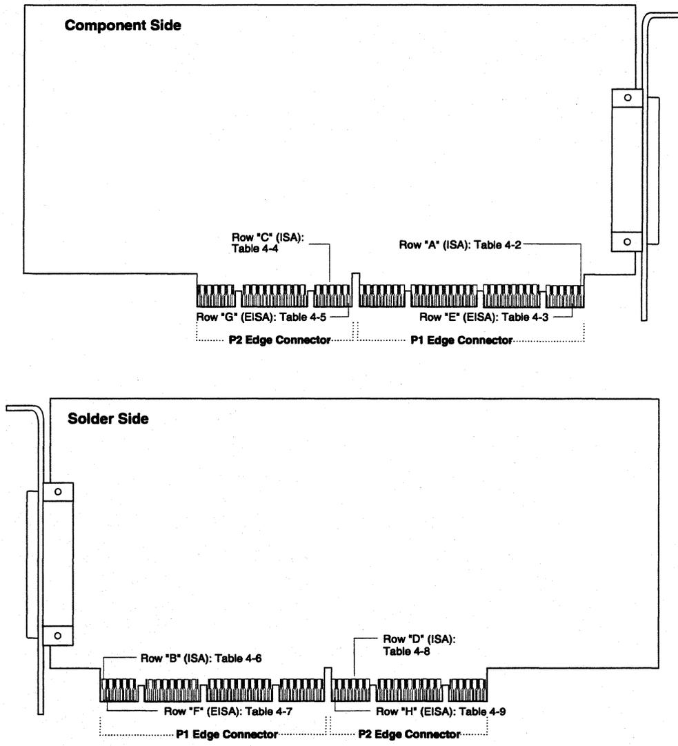
**Figure 3-4. Connector Rows on the EISA host adapter's Board Edge**
