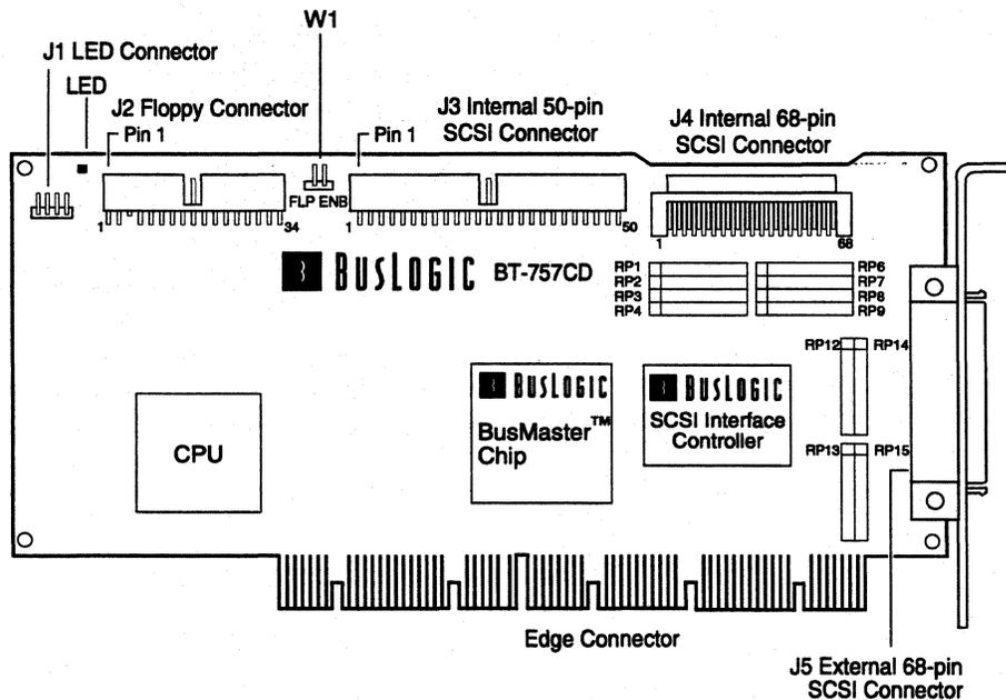
Figure 3-2. The BT-757CD Host Adapter
