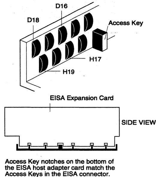
Figure 3-3. The EISA Connector/ EISA Host Adapter Interface
