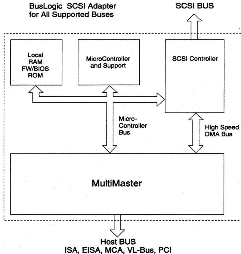
**Figure 1-1. Typical MultiMaster SCSI Adapter**
