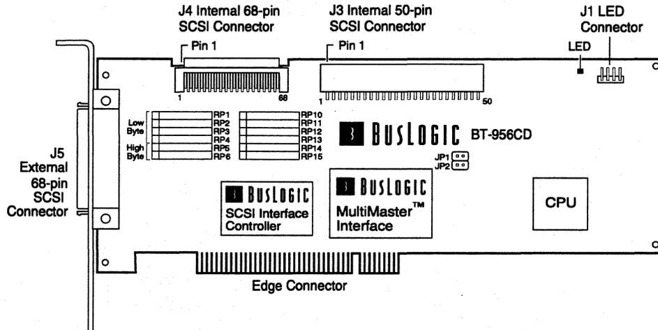
Figure 2-2. The BT-956CD Host Adapter
