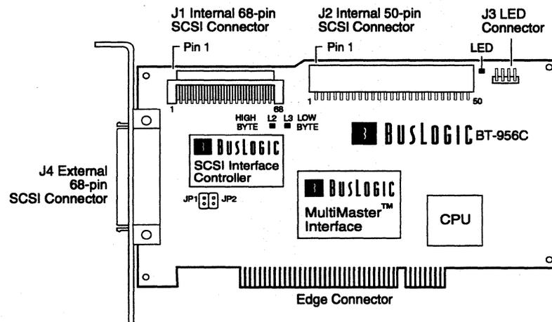
Figure 2-1. The BT-956C Host Adapter
