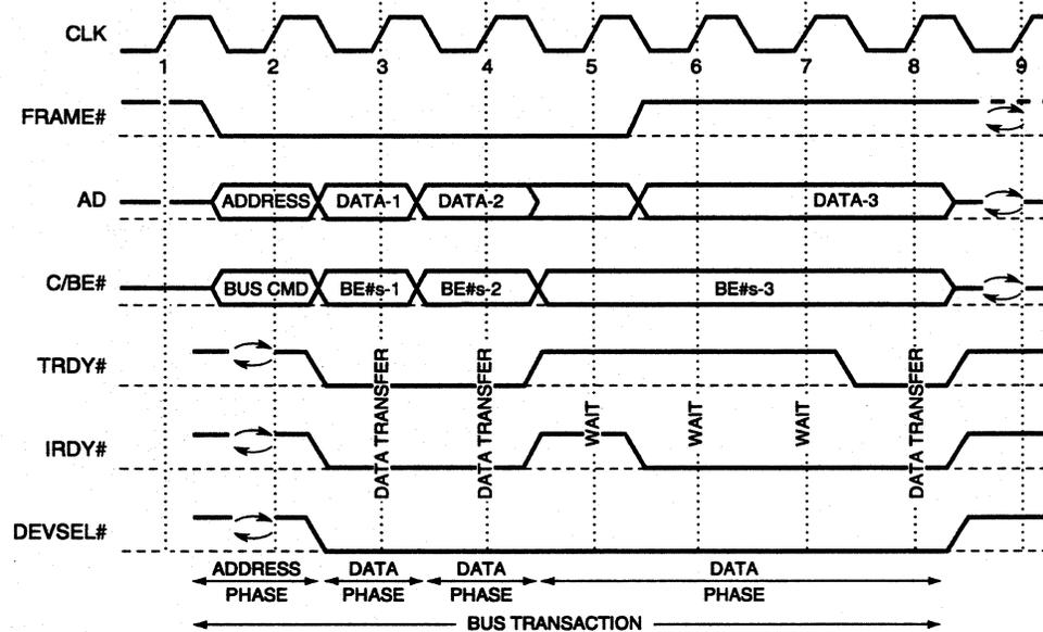
Figure 2-5. Basic Write Operation
