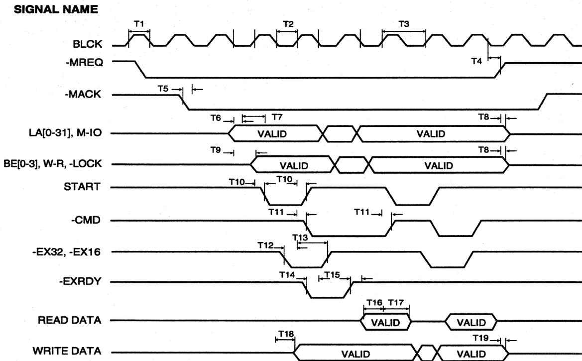
**Figure 3-5. EISA Read Cycle Timing Characteristics**
