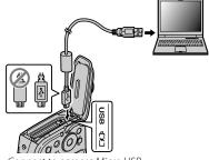
Connect to camera Micro USB connector (Micro-B)
