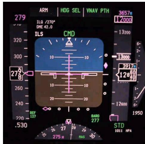
EFIS with 2 1/2 Dot ILS Deviation Figure 4
