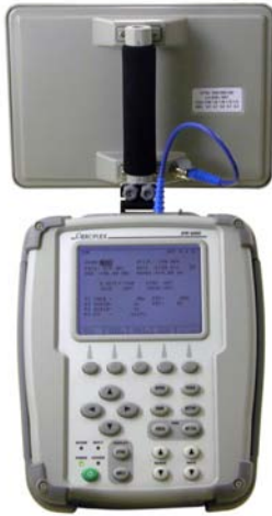
Directional Antenna Mounted on Test Set Figure 48
