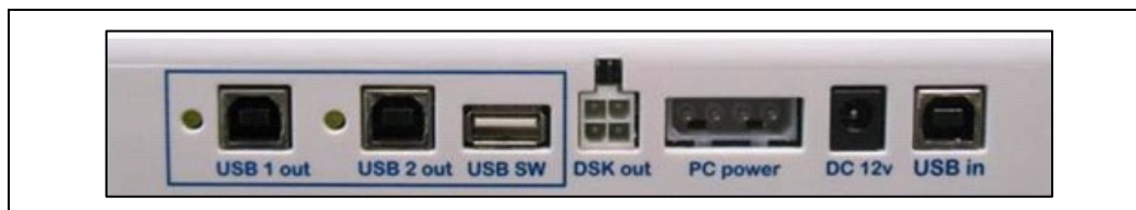
Figure 1-2. Intel® APS Rear Panel
