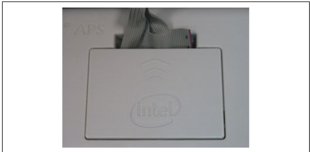
Figure 34. Feature Cable Connected to J2 (lid closed)
