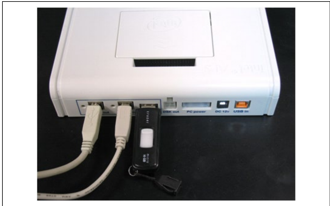
Figure 28. USB Disk on Key and 2 Computers Connected to Rear Panel
