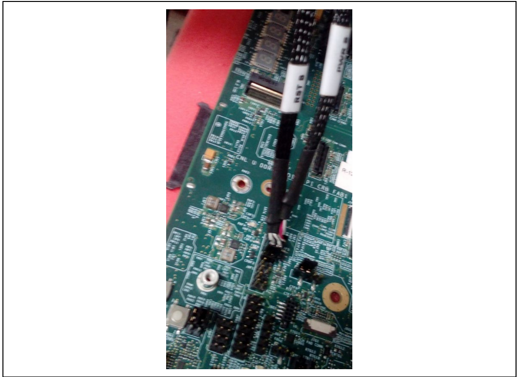
Figure 71. CFL-U Power and Reset Button Relays Connected
