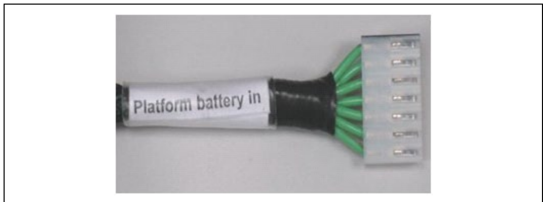
Figure 43. Molex_09-50-3081 (Intel® APS battery "IN" connector)
