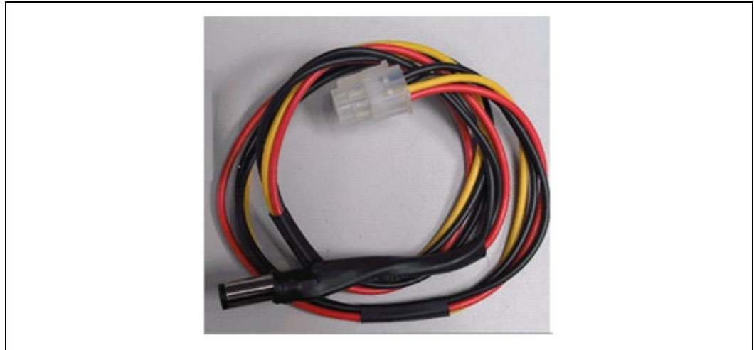
Figure 14. Section of Cut Power Brick Cable (with 4-pin Connector) that Connects to the Platform's DC Power Socket
