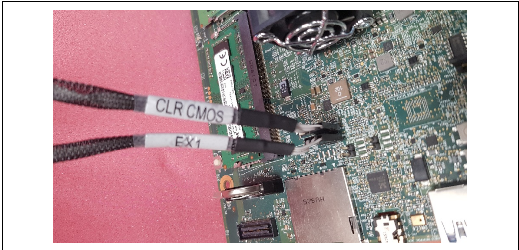
Figure 56. CLR CMOS and RTC Cables Connected to APL
