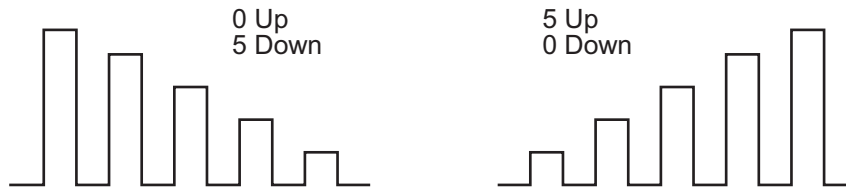
Figure 3-7 Sample one-shot only pulses for step method
