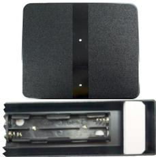
Two screws are on the bottom side of the appliance, loosen them **and the middle part can be** opened. There is a battery bracket for 4 Mignon Batteries. Look for the correct polarity. Pull the batteries slowly out of the bracket and set in the new batteries. Then put it back and screw the middle part back onto the electrode.
