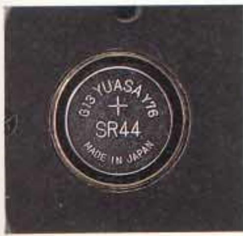
Battery Chamber Contains two SR44 silver or LR44 alkaline batteries.
