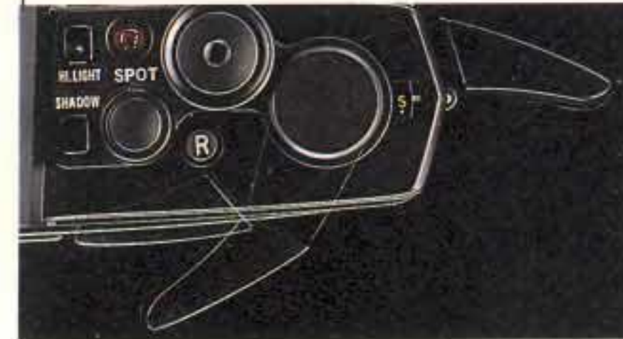
SPOT Metering Button Just a touch of this button, and you have automatically taken your first spot reading — as well as setting the camera for Multi Spot mode. You can keep pushing it as many times as you like until you are absolutely satisfied you have the exact exposure selection you want. Each time a new spot appears on the finder display, and the last eight spots are automatically calculated for the final exposure value. Audio indications can be switched on or off.
