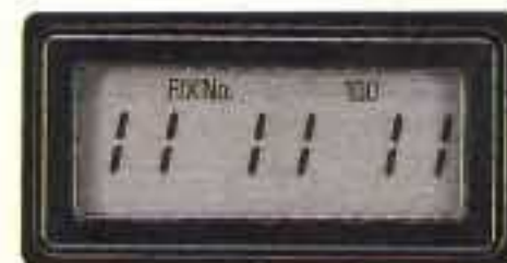
Fixed Code. Alternatively, the Recordata Back 4 can be programmed to imprint a fixed code directly on the photograph. The code selected and preset will then appear on all the frames shot, until the Recordata Back is reset.
