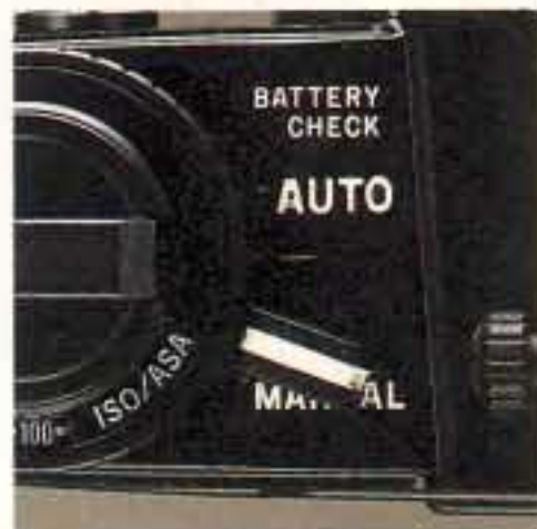
Mode Selector Lever Switches the camera between Manual and TTL Direct Auto modes, and also provides an audio-visual battery check position. Multi Spot exposure readings can be made with the camera in either Auto or Manual modes.
