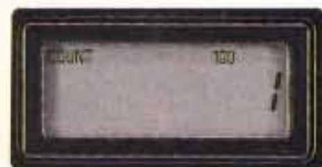
Frame Counter. Up to six digits can be selected freely to form a desired code for the frame counter. This will advance one digit with each frame, establishing a sequence for the pictures taken.
