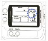
Note: The guide number (GN) automatically changes according to the shutter speed.
