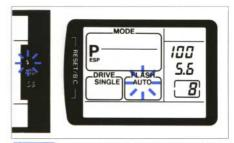
Make sure AUTO lights on the LCD panel. When the flash is recharged, \$\forall \text{ in the viewfinder will light.}
