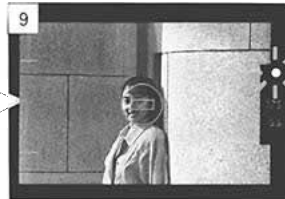
9 Depress the shutter release button halfway, making sure the autofocus indicator in the viewfinder lights and the autofocus beep is heard (p. 20).
