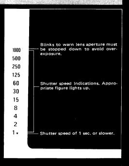
The OM-PC also provides manual exposure control. With the exposure mode dial set to MANUAL, you can choose your desired aperture and shutter speed combination. You will see the following display in the viewfinder.
