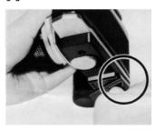
2) Carefully push the Motor Drive Plug forward and up until It snaps into the front of the Motor Drive 1.
