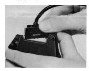
Push the Power Supply Plug down until it snaps into the front of the Control Grip.
