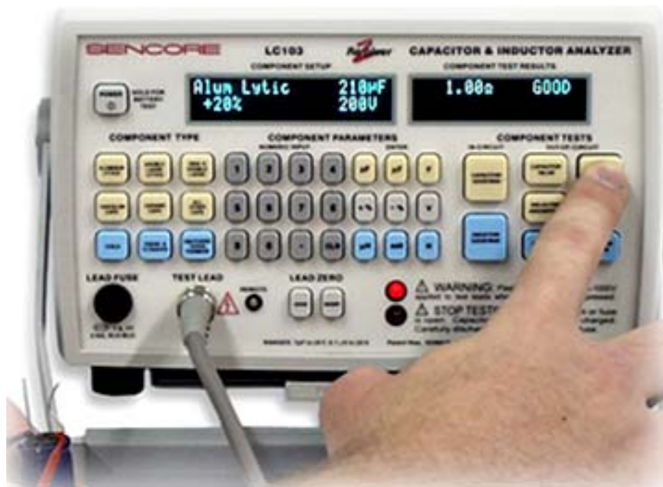
Figure 7. Each Z-meter test indicates good or bad, eliminating any chance of interpretation or calculation errors.
