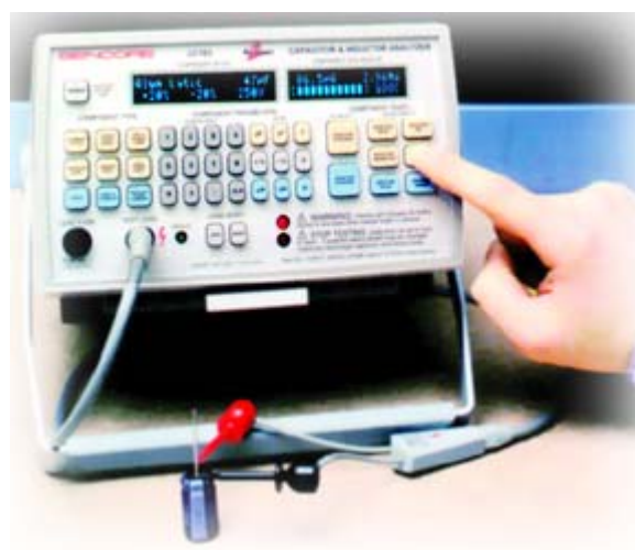
Figure 6. The Z-Meter's programmable leakage power supply tests leakage on any capacitor at its working voltage up to 1000 volts.
