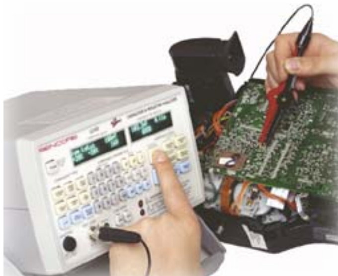
Figure 9. The LC103 in-circuit capacitor test indicates capacitor value and ESR after performing a series of in-circuit analyzing tests.
