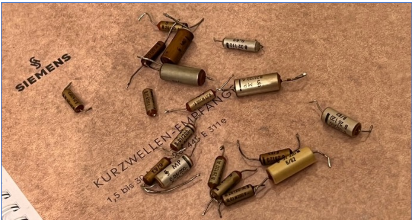
Some of the replaced MP capacitors
