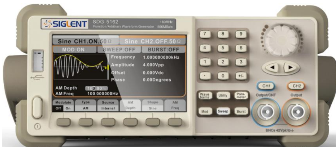
Figure 1- 2 Front Panel of SDG5000 Series
