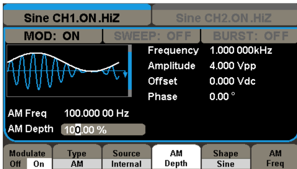
Figure 1- 15 Modulated Waveform Display Interface
