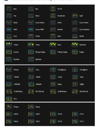
Parameter measurements includes 4 categories: horizontal, vertical, miscellaneous and CH delay providing a total of 50+ different types of measurements. Measurements can be performed within a specified gate period. Measurements on Math, Reference and History frames are supported
