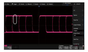
With a waveform update rate of up to 110,000 wfm/s, the oscilloscope can easily capture unusual or low-probability events. In Sequence mode the waveform capture rate can reach 500,000 wfm/s
