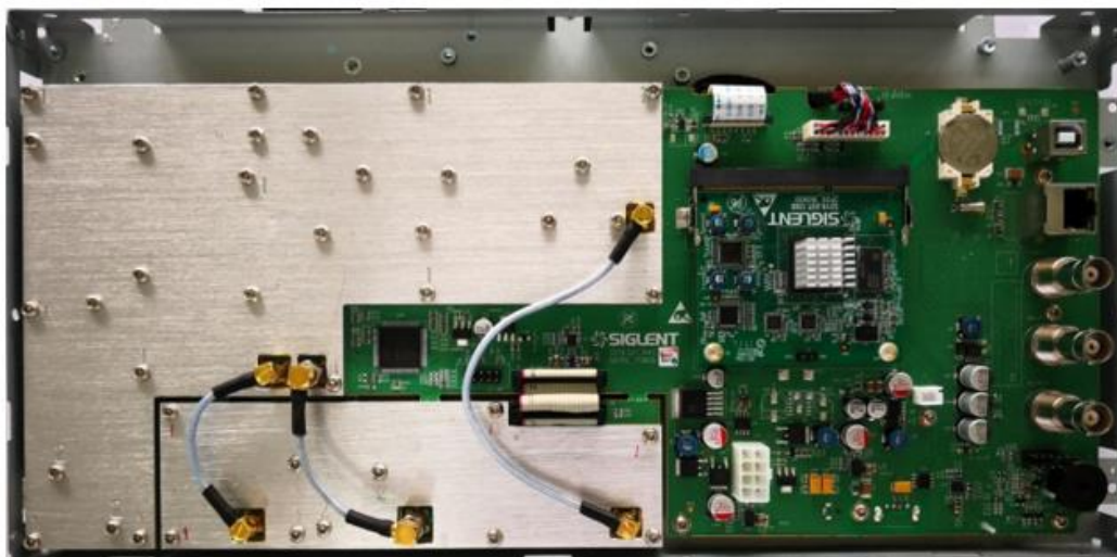
Figure 4-4 View of front panel subassembly with the mainboard
