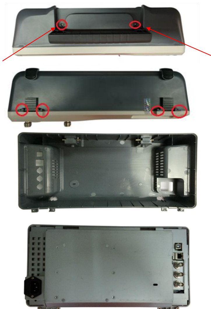
Figure 4-1 Removing the Rear Panel Screws
