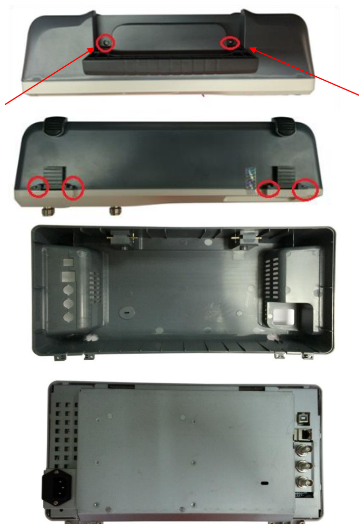
Figure 4-1 Removing the Rear Panel Screws
