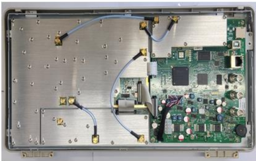
Figure 4-4 View of front panel subassembly with the main board
