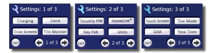
Use the Setting screens to change various vehicle behaviors and Touch Screen features. For example, you can change charge settings, specify the drive screens that are displayed, set a security PIN, program a button on your key fob, and prepare your vehicle for safe transportation (see the Roadside Assistance Guide, provided in the owners package, for details on how to safely transport the vehicle).
