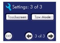
4. Touch **Tow Mode**, then touch **OK** to confirm. The Touch Screen displays the following message indicating that the vehicle is in Tow Mode.
