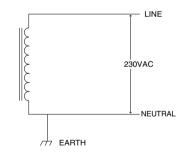
Caution: The LINE connection must measure 230V RMS to NEUTRAL. EARTH must also be connected to the Home Connector.
