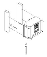
2. Attach the Home Connector to the wall studs using four  $1/4" \times 2 1/2"$  (M6) lag screws. The length of the screws must be adequate to securely anchor the Home Connector.
