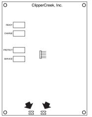
Two "Charge Test" buttons on the PC board (arrowed in illustration) simulate connection to a vehicle.
