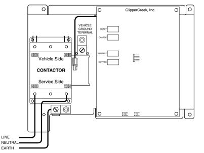
To access the electrical connections, open the enclosure by removing the two screws on the left-hand side using a T15 Torx L driver. Then unhook the latch located on the bottom of the unit (over the cable holder). Caution: Before connecting any wires, make sure you have identified the type of utility service connection available. For more information, refer to Utility service connections, page 4.
