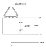
Caution: Do not use a 3-phase delta-connected transformer secondary without a center tap on one leg. No "neutral" point is available for the required ground connection.
