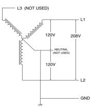
With a wye-connected secondary, any two of the legs can be used to provide 208V to the Home Connector. For example, L1 and L2, or L1 and L3, or L2 and L3.
