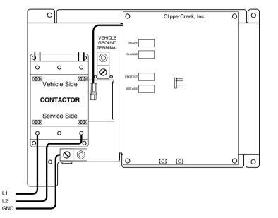
To access the electrical connections, open the enclosure by removing the two screws on the left-hand side using a T15 Torx L driver. Then unhook the latch located on the bottom of the unit (over the cable holder). Caution: Before connecting any wires, make sure you have identified the type of utility service connection available. For more information, refer to Utility service connections, page 4.
