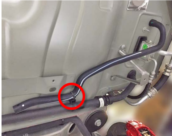
✓ Figure 1 (Drain hose correctly installed)
