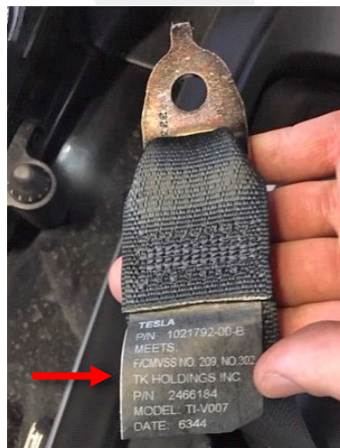
Figure 1 (Correct label on replaced part)
