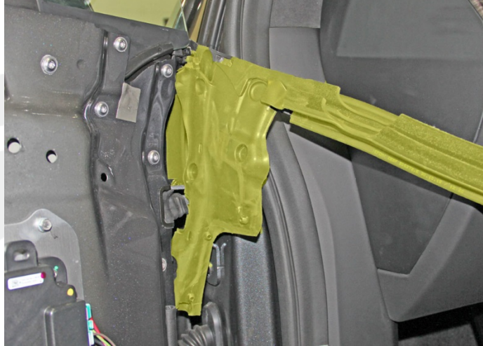
Figure 2 (Inner belt seal highlighted)
