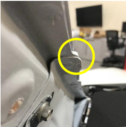
Figure 3 – Uneven sheet metal overlap, edge view
