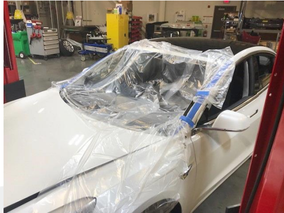
Figure 5 – Mask work area and protect IP carrier and interior
