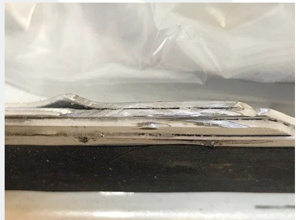
Figure 7 – Sheet metal layers ground flush
