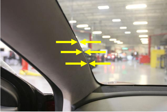
Figure 1 – Bulge from inside
