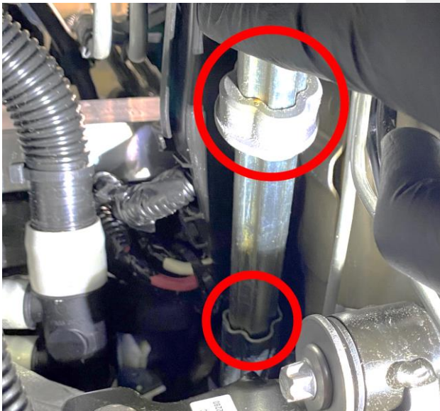
✘ Figure 2 – Steering column shaft joint exposed
