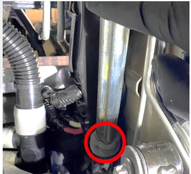
✔ Figure 3 – Steering column dust cover installed on the steering column shaft joint
