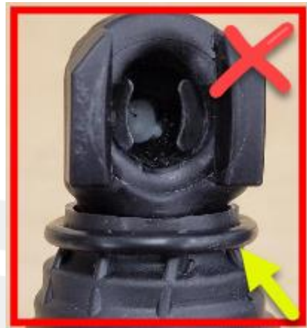
Figure 4 - O-ring seated too low
