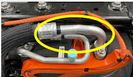
Figure 3- Foam Not Installed (Europe)
