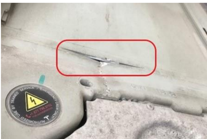
Figure 6 – Visible open crack
