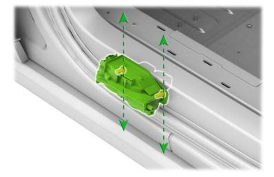
The striker can be adjusted to move the rear door along the X-axis (forward or back) and the Y-axis (in or out).
