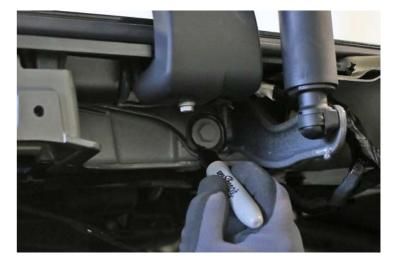
With the upper door in the open position, loosen the bolts that attach the hinges to the spine.
