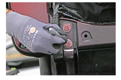
With the upper door in the open position, loosen the bolts that attach the hinges to the door frame.
