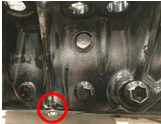
Figure 12 – Skid plate to doubler fastener sheared/bent
