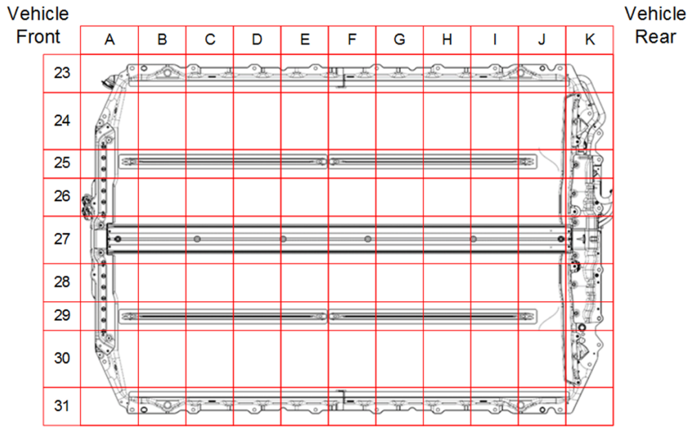
Figure 4 – HV battery grid layout
