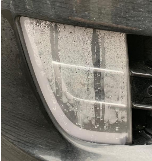
Figure 5 Unacceptable fascia (fog) light water ingress
