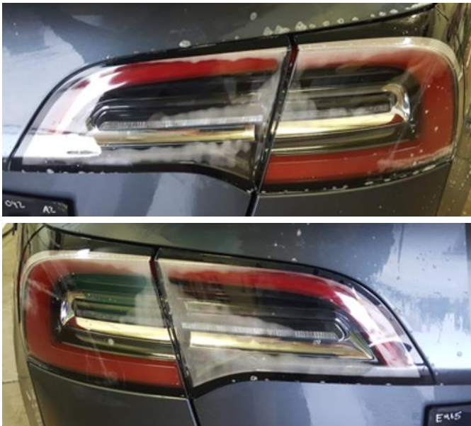
Figure 3 Acceptable taillight condensation
