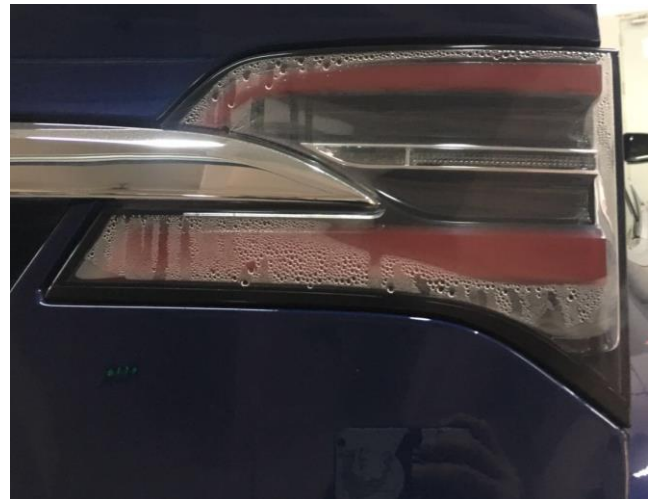
Figure 8 Unacceptable taillight water ingress
