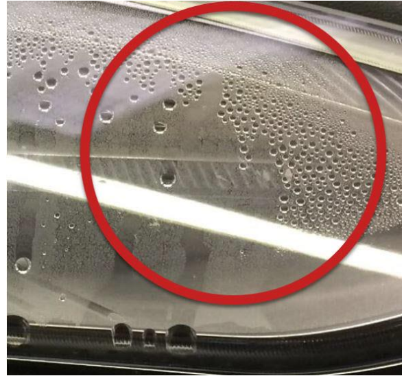
Figure 6 Unacceptable headlight water ingress
