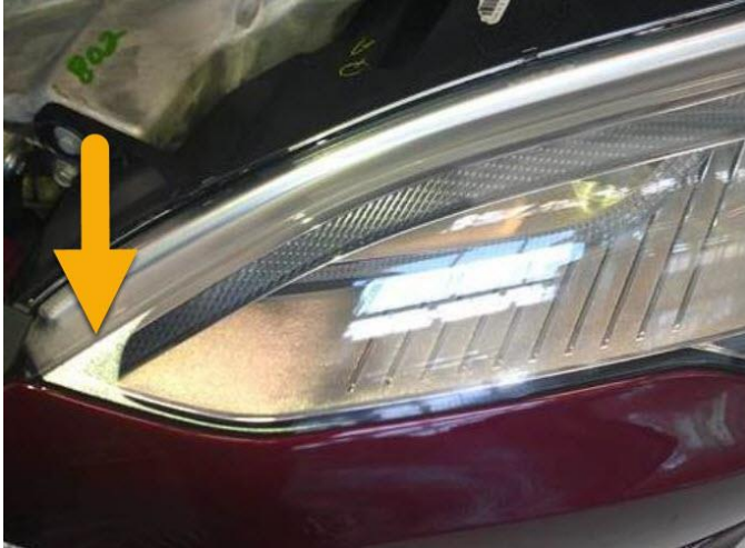
Figure 1 Acceptable headlight condensation
