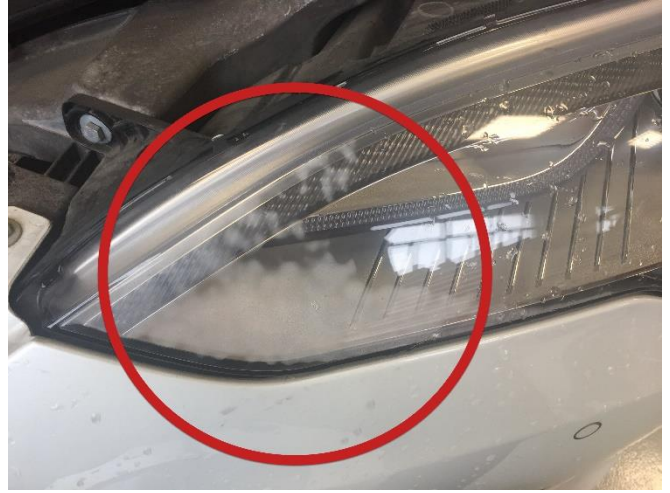
Figure 2 Acceptable headlight condensation
