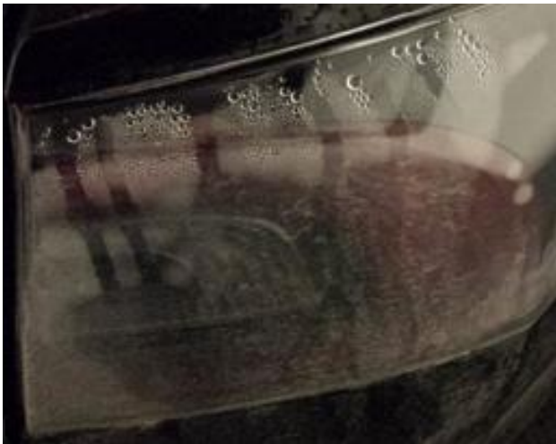
Figure 7 Unacceptable taillight water ingress
