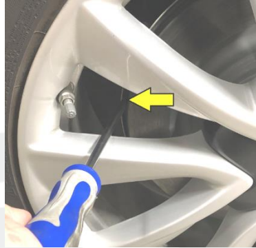
Figure 3 – also push on the right side of the shield, if necessary
